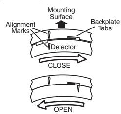
• **Removal**: Depress tab with a small slotted screwdriver. Rotate detector counter-clockwise until the alignment marks line up. Remove detector.
