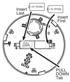
If batteries are not installed, install batteries in the sequence indicated. Use only approved Panasonic CR123A, Sanyo CR123A or Duracell DL123A batteries. If batteries are installed, remove the 'Pull' tab to activate.
