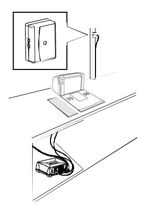
Wireless synchronization modules can significantly reduce electrical interference between Sensormatic EAS systems timed to the AC line. A module system includes a module designated as a transmitter and one or more modules designated as receivers.
