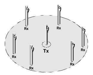
Receivers (Rx) must be within 60.1m (200 feet) of the transmitter (Tx)
