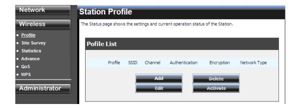
Configure the setting to connect to a wireless network, selection option for network type, SSID, and wireless security. The profile can be edited, deleted and made active from this option.
