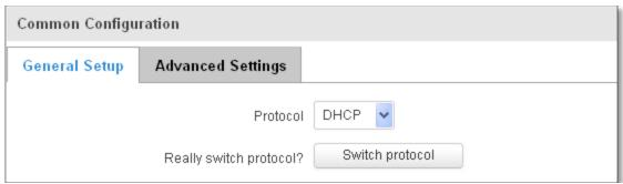
You can switch between the Static, DHCP or PPPoE protocol by selecting the protocol that you want to use and then pressing **Switch Protocol**.
