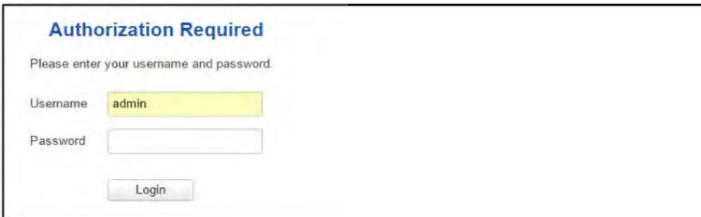
Enter the default password, which is "admin01" into the "Password" field and then either click Login with your mouse or press the Enter key. You have now successfully logged into the RUT955!
