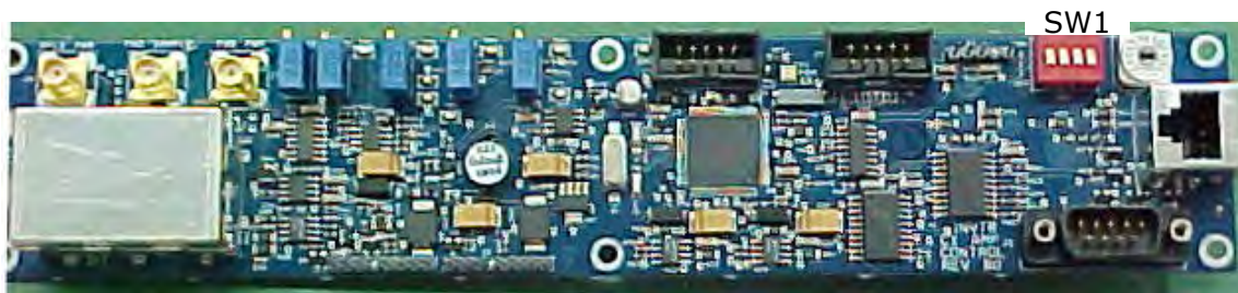
Amplifier Control Board
