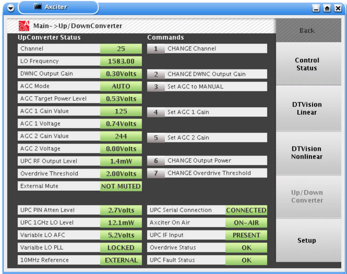
Figure 5-1: Axciter Upconverter/Downconverter Main Screen
