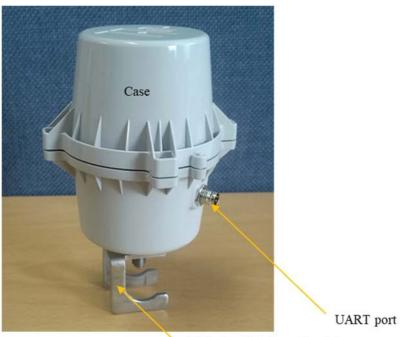
Fixing bracket for water piping
