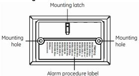
B. Insert the two screws provided and secure the mounting plate to the wall or ceiling surface. (If mounting in plasterboard or
