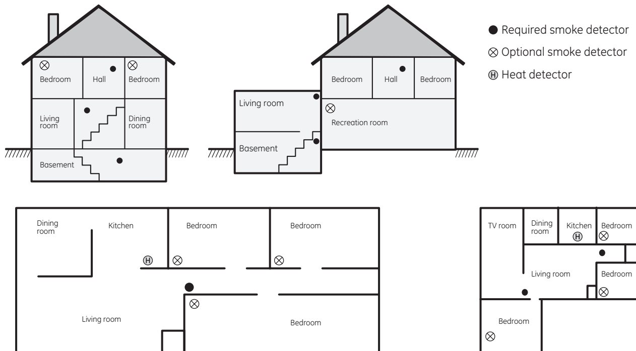
Figure 5. Smoke detector locations
