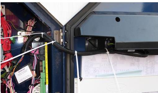
**12** If there is RMM: Take out the green RMM power connector and replace it with ArrowTrack connector
