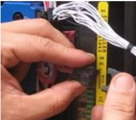
**4** Take out the green RMM power connector and replace it with ArrowTrack connector
