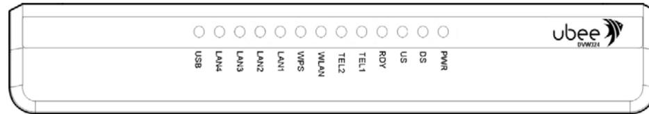
Figure 4: Front Panel LEDs
