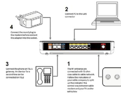
Figure 3: Connection Diagram
