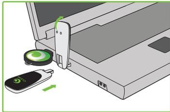
\*Right Angle Connector is needed when inserting the Clear USB into a vertical USB slot.
