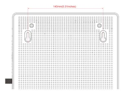
**Note:** The screws should protrude from the wall so you can fit the device between the head of the screws and the wall. If you install the screws in drywall, use hollow wall anchors to ensure the unit does not pull away from the wall due to prolonged strain from the cable and power connectors.
