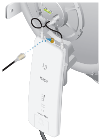
Connecting the GPS Antenna
