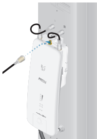
Connecting the GPS Antenna
