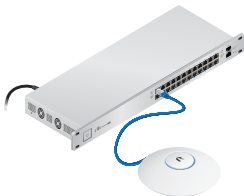
UniFi Switch Power Connection Diagram
