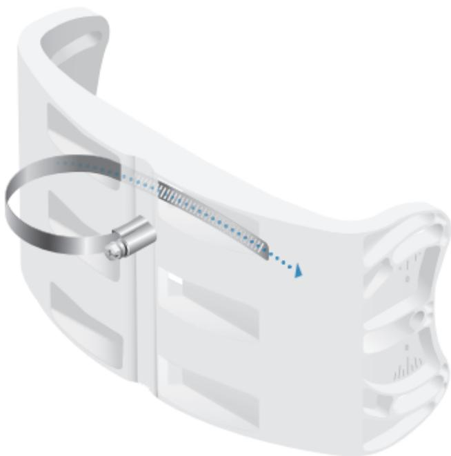
2. To mount the *Mounting Bracket*, wrap each *Metal Strap* around the pole. Use a 7 mm socket wrench or screwdriver to turn the screw clockwise and securely fasten the strap to the pole.
