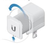
3. Slide the outer casing back onto the adapter until it snaps into place.
