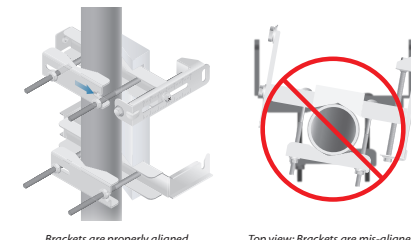
Brackets are properly aligned. Top view: brackets are mis-aligned.
