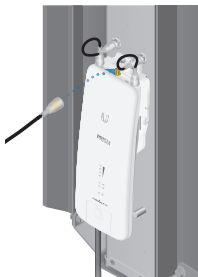
Connecting the GPS Antenna
