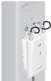
Connecting to a Sector Antenna
