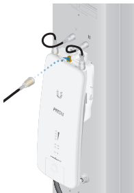
Connecting the GPS Antenna
