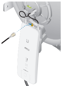
Connecting the GPS Antenna
