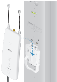
Mounting on a Sector Antenna
