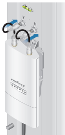
Connecting to a Sector Antenna
