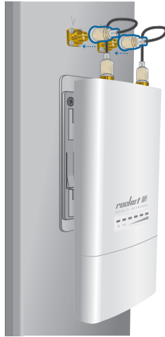
Connecting to a Sector Antenna
