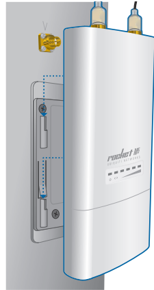
Mounting on a Sector Antenna
