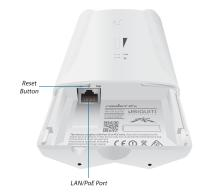
**LAN/PoE** This Gigabit Ethernet port is used to connect the power and should be connected to the LAN.
