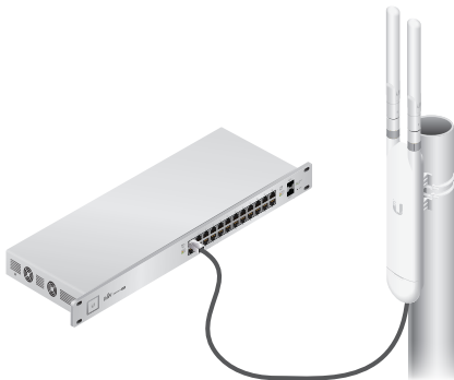
Connected to UniFi Switch, model US-24-250W
