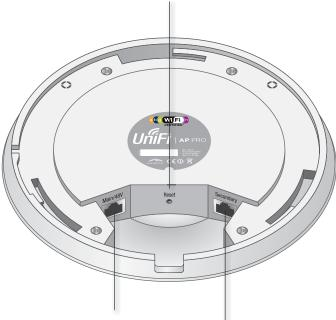
Main/48V The 10/100/1000 Mbps port connects the power and should be connected to the LAN and DHCP server. Power can be provided by a 48V, 802.3af compliant switch or by the included PoE adapter.
