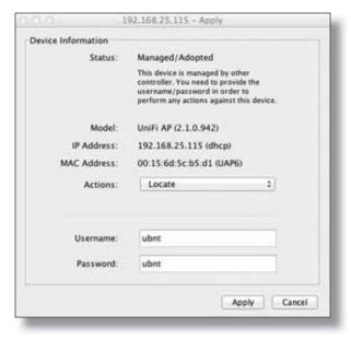
The LED on the Access Point will flash so that it can be identified from other Access Points. If the Access Point's status requires the entry of a username and password, enter them before clicking *Apply*.
