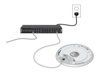
802.3af Switch Power Connection Diagram
