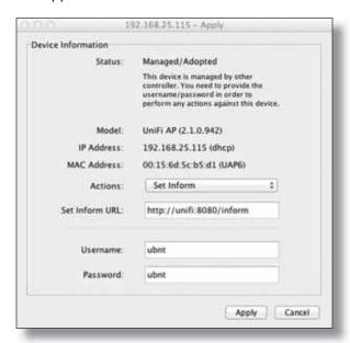
Enter the URL, port, and path to the instance of the UniFi Controller software that the Access Point is to be managed by. If the Access Point's status requires the entry of a username and password, enter them before clicking *Apply*.
