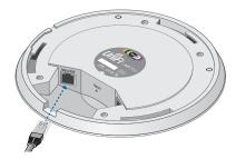
7. Align the notch on the UniFi AP-Pro with the notch on the *Mounting Bracket*.
