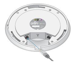
6. Align the notch on the UniFi AP-Pro with the notch on the *Mounting Bracket*.
