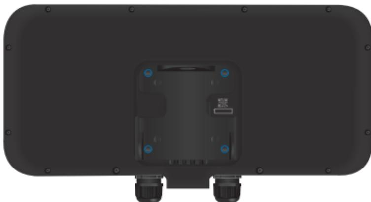
The 8-hole mounting pattern on the back of the UAP-StadiumXG follows the VESA MIS-D standard and can be used with mounts that comply with this standard. Use either the 100 x 100 mm or 75 x 75 mm square hole pattern with M4 x 10 screws.
