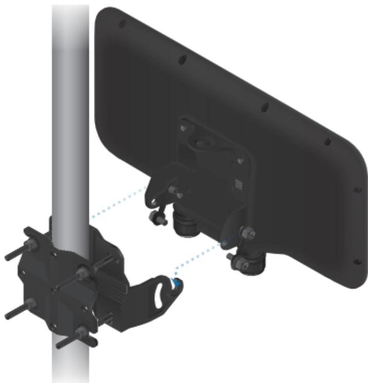
5. Insert the *Elevation Lock Bolts* into the adjustment slots. Remove the lanyards and then tighten the bolts by hand.
