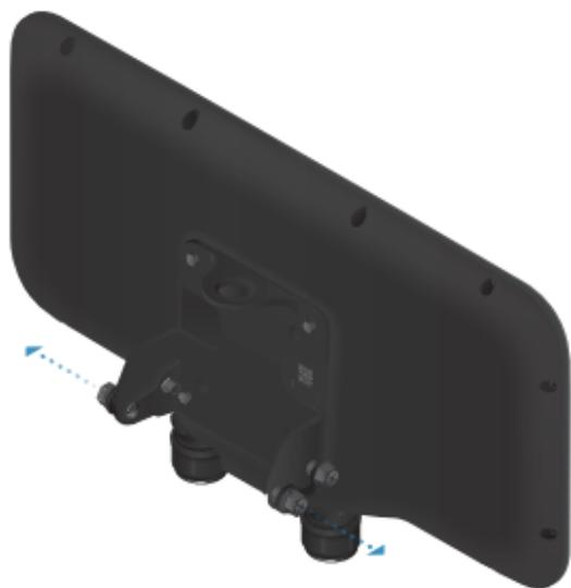
7. Lift the UAP-StadiumXG and align the *Mounting Bolts* with the slots on the *Adjustment Bracket*. Seat the *Mounting Bolts* in the slots.
