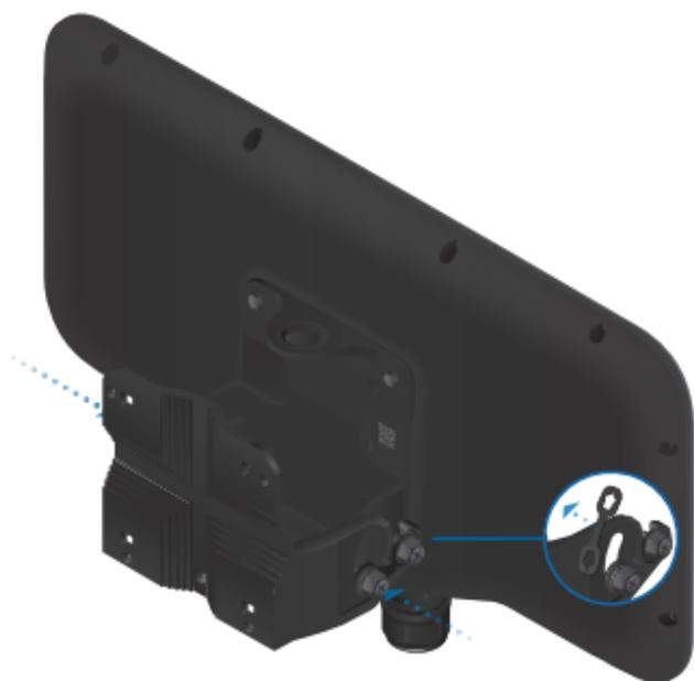
9. Pivot the UAP-StadiumXG until it reaches the desired elevation angle (+10 to -50°). Then tighten all bolts.
