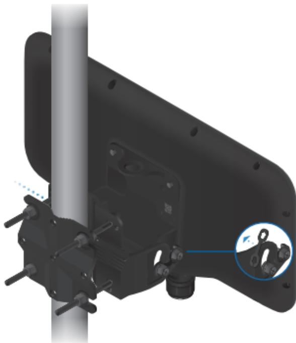
6. Pivot the UAP-StadiumXG until it reaches the desired elevation angle (+10 to -50°). Then tighten all bolts.
