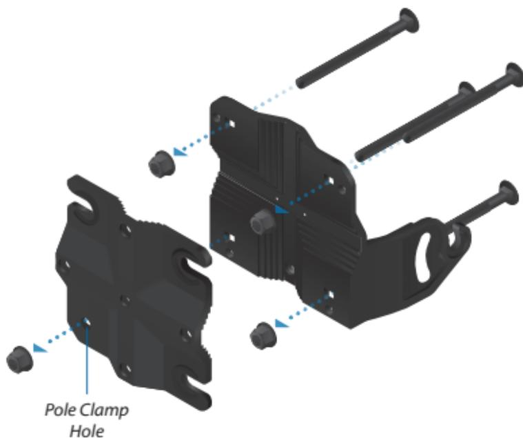
2. Mount the *Adjustment Bracket* on the pole and secure it.
