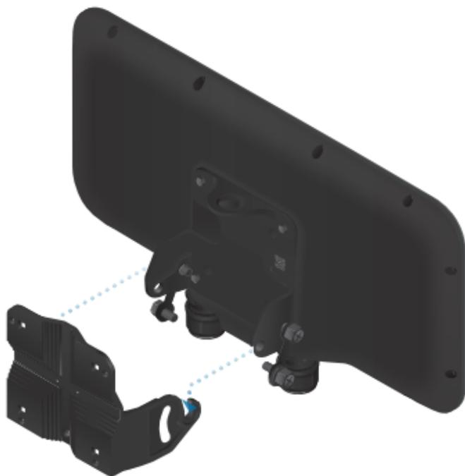
8. Insert the *Elevation Lock Bolts* into the adjustment slots. Remove the lanyards and then tighten the bolts by hand.
