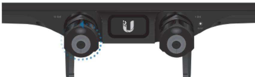
2. Remove the plug from the grommet.
