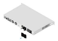
2. Insert the PSU module until the *Lock Lever* engages and locks into place.
