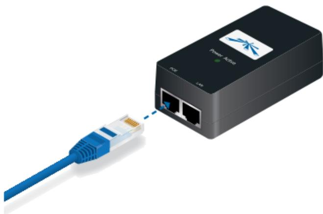
3. Connect an Ethernet cable from your LAN to the Ethernet port labeled **LAN** on the *PoE Adapter*.
