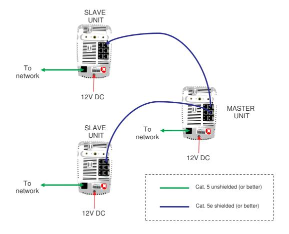
WARNING: Never plug a networking cable into a timing cable socket, or a timing cable into the networking socket!
