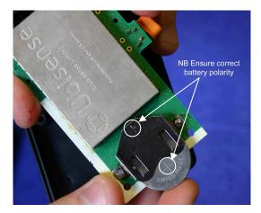
When both batteries have been replaced, the Ubitag will bleep once and flash its LEDs to indicate correct start-up, and the Ubisense In-Building Location System will then be able to determine the Ubitag's location. Replace the back of the Ubitag and tighten the four screws removed previously to complete reassembly of the device.
