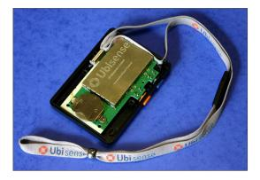
To remove the mounting cord, undo the retaining screws on the back panel of the Ubitag (as shown above in the section 'Replacing the batteries in the Ubitag'), remove the panel, and detach the mounting cord. Replace the back of the Ubitag and tighten the four screws removed previously to complete reassembly of the device.
