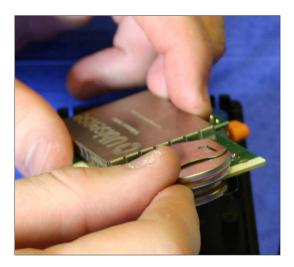
Leave the Ubitag unpowered for 30 seconds, then insert two fresh batteries into the retainers, observing the polarity marked on the battery and the retainers:
