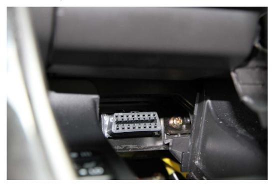
Most of the OBD port located in the driver side and under of the dashboard or near the walking box as above picture showed.
