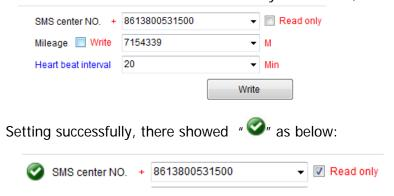
**Note:** When inquiry and setting SMS center No., the 3G module must be at work status. Hence the device must be powered from OBDII port and the working time of 3G module should be more than 15s.
