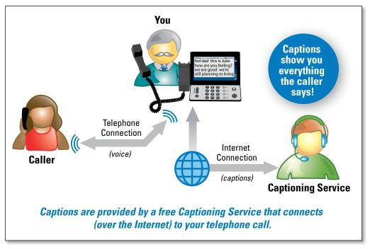
Your new CapTel 2400i works like any other phone – just pick up the handset and dial the person you want to call on the dialing keypad. Every time you make a call, the phone can also connect over the Internet to a free Captioning Service. An Operator at the Captioning Service uses speech-recognition technology to create captions of everything your caller says. The captions appear on your CapTel 2400i display screen for you to read.
