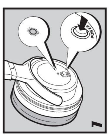
Switch on the headphones and make sure the running light comes on; this confirms that the rechargeable batteries contain power. Turn the volume adjustment thumbwheel to the half-way position.
