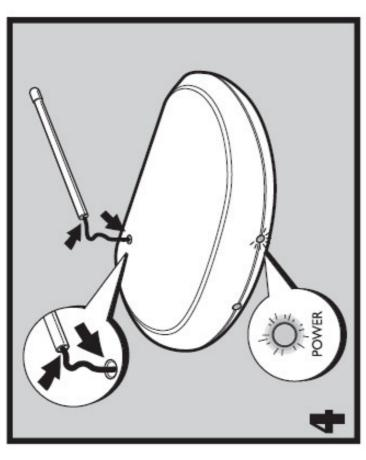
The **Green** running light comes on when the transmitter is connected to the audio source and the audio source is turned on.
