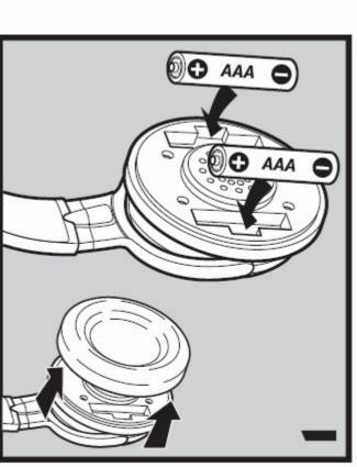
Open the rechargeable battery compartment on the right side (R) of headphone receiver, and insert two AAA type rechargeable batteries as enclosed in the packaging of the product, making sure their positive and negative (+ and -) poles are correctly aligned.
