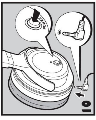
GB After using the headphones, switch them off and connect them back up to the transmitter using the cable with the 2.5mm power jack, thereby recharging the rechargeable batteries.
