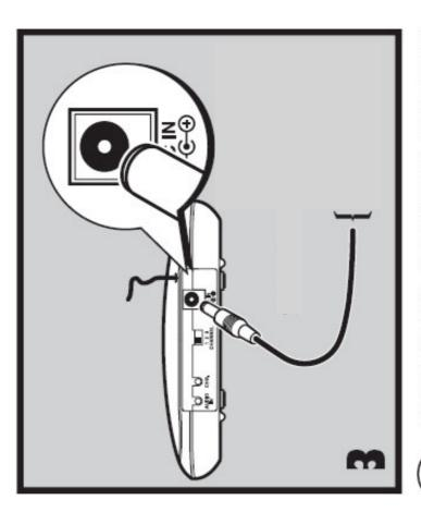
GB Connect the plug on the AC/DC mains adapter cable to the DC IN socket at the back of the cradle then plug the adapter into mains wall outlet.
