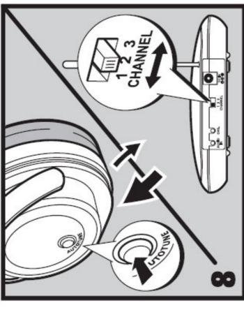
(GB) Adjust headphone reception by pressing the auto scan button. If the sound is poor, change to a different channel on the transmitter and press the auto scan button once more.
