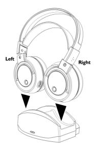
3. The charge process starts automatically and the green Charging Indicator light comes ON. Be sure to charge new batteries before using them for the first time. The green indicator light will be ON during the charging process, and will turn OFF when batteries are fully charged.
