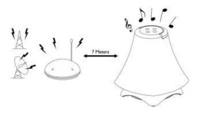
5. You should now be able to place the speakers freely from room to room without disruption. Should there is any disruption (signal cuts off or carries distortion), press the speaker's "AUTO TUNE" button to maximize the best reception.
