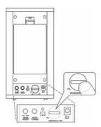
Switch on the speakers by turning up the VOLUME ON / OFF knob towards ON direction. The POWER / STEREO LED will light up. Switch off the speakers by turning down the VOLUME ON/OFF knob towards OFF direction until a "click" sound is heard.
