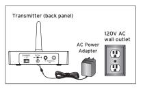
Connect the small, round plug from the transmitter AC power adapter to the transmitter's DC IN jack. Plug the other end of the transmitter AC power adapter into any standard 120V AC wall outlet.
