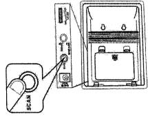
A). Keep a distance of the speaker up to 7 meters apart from transmitter, and then press "SCAN" auto-tuning button for best tuning reception.
