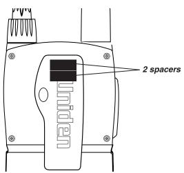
Warning: Do not operate your ATLANTIS radio when using the optional Speaker/Microphone unless both spacers are properly affixed behind the beltclip.
