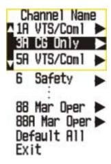
Pressing the UP or DOWN arrow keys will scroll through a list of preprogrammed channel names. A selection of Default all, when selected, will restore all of the channel names to the factory default channel names.
