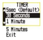
From this screen, the user can select how long the backlight stays on after any key press or if the Light / Lock key is momentarily pressed. Select Exit will return the radio to the Lamp Adjust menu.
