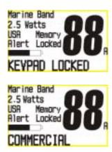
The only keys and controls that can be used in this mode are the PTT key, Light/Lock key, 1/2.5/5W key, Volume, and Squelch. To deactivate the keyboard Lock function, hold down the Light/Lock key for 2 seconds and the Locked text will disappear, or turn the radio off and back on again. The keyboard lock function will not remain in memory
