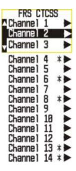
Using the UP or DOWN arrows keys, the user will select a channel to assign a CTCSS code to. Channels that have an asterisk after the channel numbers indicate that these channels currently have CTCSS codes assigned to them.
