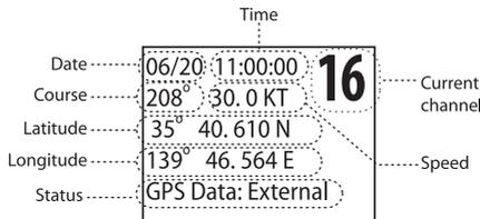
If the GPS does not send coordinates within 30 minutes, an audible alert sounds once and the display shows *Input GPS*. This message remains until the coordinates are updated.
