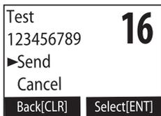
5. The radio automatically switches to channel 70 to transmit the test call request, then switches back to the last-used channel.
