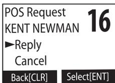
To send your current position to the other station, select *Reply*; the radio transmits your latitude and longitude to the other station. If you select *Reply* but the radio does not have valid GPS data, it transmits the reply code with *No Position*.
