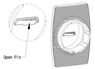
4. Insert the emergency opening pin into the emergency opening hole.
