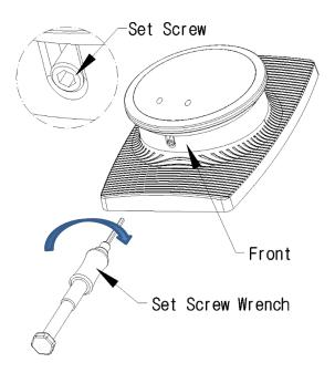
2. Rotate the front bezel to clockwise and take out the front core.
