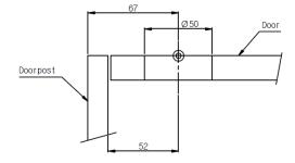
Note 1 : Bracket position is depend on the door thickness. Note 2 : Cut off the marking point of the bracket.
