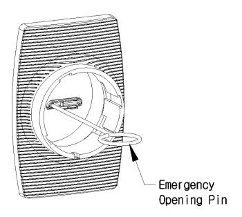
• The lock does not work at all after this emergency opening. Return the lock to the authorized dealer for rework.
