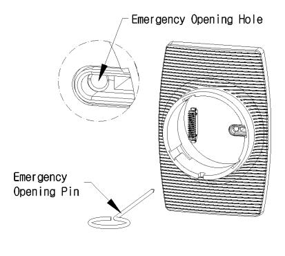
5. Press the emergency opening pin to the right end and open the door.
