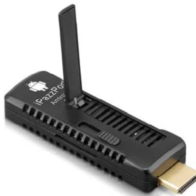
**3.3 input device:** This device support standard USB keyboard and mouse, also support RF 2.4G Voice Wireless keyboard. Left mouse for click, right mouse for back.
