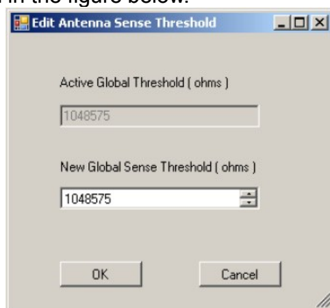
Antenna Sense Threshold Settings
