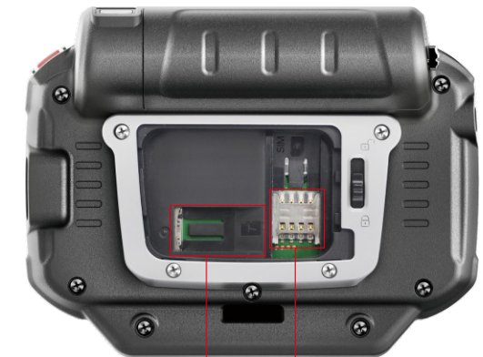
Micro SD/TF Slot Micro SIM Slot
