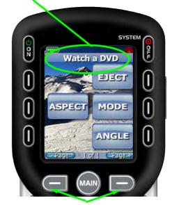
Press either of the PAGE buttons to see other Screen buttons for this device. Any of the buttons can be custom labeled.
