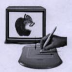
Erasing. In supporting applications, the pen's eraser works like the eraser on a pencil. In text applications, use the eraser to select text. then lift the eraser from the tablet to delete the text.
