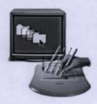
Using the Graphire 2 Cordless Mouse. Place the Cordless Mouse on the tablet. The screen cursor is positioned when you move the Cordless Mouse across the tablet surface. Move the fingerwheel forward or backward to scroll in the active window.
